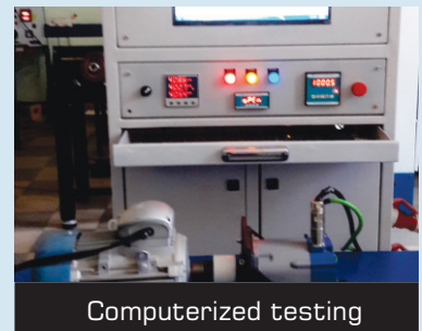
Surge and leakage Current testing
